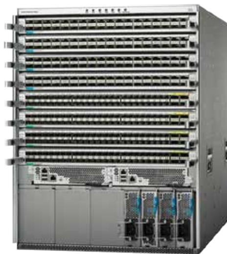
Campus Core block will be used to route traffic between multiple blocks i.e. traffic across multiple block has to transit through the Core network. Two Cisco Nexus 7710 switches will be used as Core switches, which will have dual 40Gig connectivity to DC Core Switches and multiple distribution blocks.
